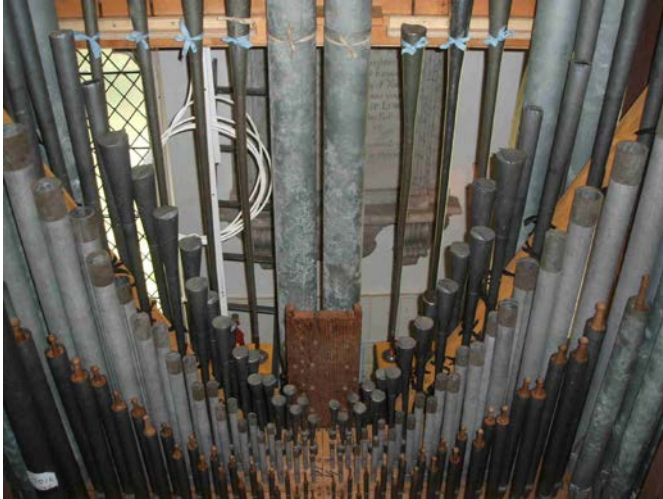
(above) Rear Swell pipes replaced with slender conical Contra-oboe pipes at the very back
