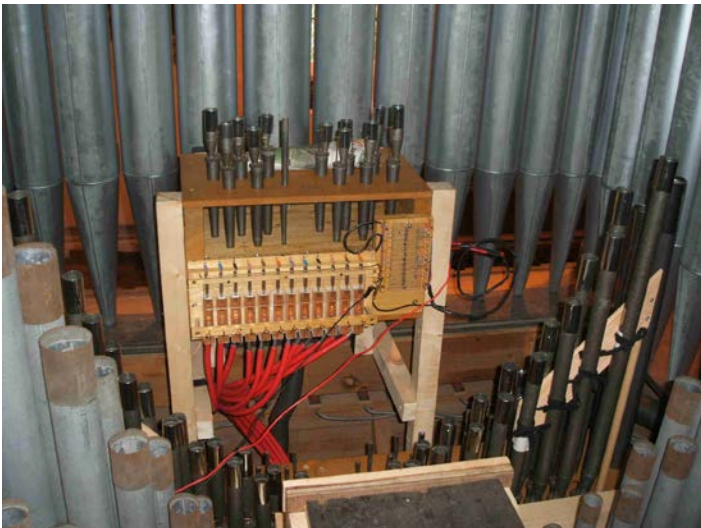
(below) the Great Organ after cleaning with new Clarinet in place (top octave on its own electric chest)
